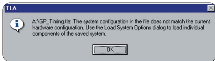
▶ Figure 3-3: Information window asking user to use "Load Systems Options" dialog to configure setup on new logic analyzer.
